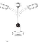
Adjust the range of the light: When adjusting the angle of the hose, please press the base of the lamp at the same time, the hose can adjust the angle freely (overadjusting the active joint part of the product will result in joint function damage)
